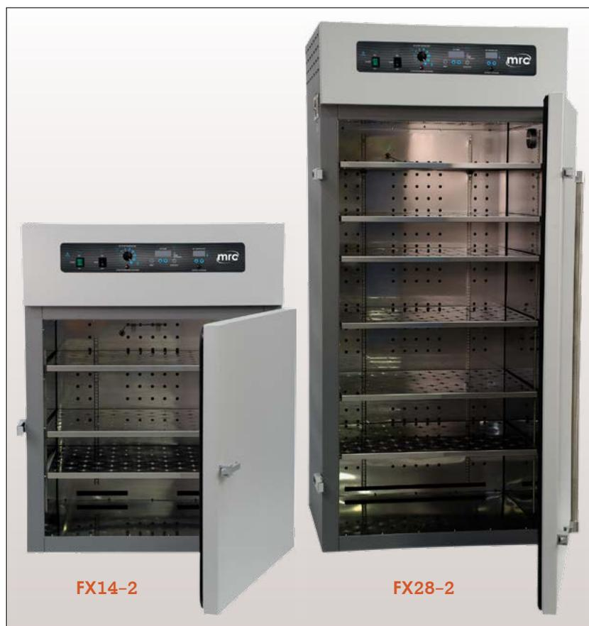
The MRC forced air ovens feature 13 or 27 cubic feet of economical oven space. The forced, blower-assisted airflow design offers excellent temperature uniformity and fast recovery. A turbo blower and heavy-duty motor combine to direct air over the shelves and samples for even, constant drying, curing and baking. These units are especially ideal for glassware drying.
